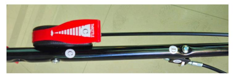
4. Using the screws supplied, losen the tape and fasten the throttle lever "C" and cable thunb wheel "D" on the Outer Left hand side of the handle as shown.
