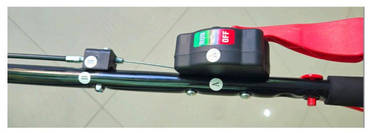
2. Using the screws supplied, fasten the reel clutch lever "A" and cable thunb wheel "B" on the Outer Right hand side of the handle as shown.
