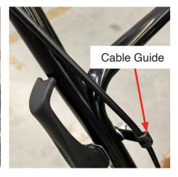
1. Open the box and remove all the packaging, but leave the mower on the pallet. Fit the lower handle using the screws and nuts provided. Fit the upper handle to the lower handle with the levers pointing upwards, as shown above. Make sure to fit the cable guides. Cable "A" on the Right and "C" on the Left.
