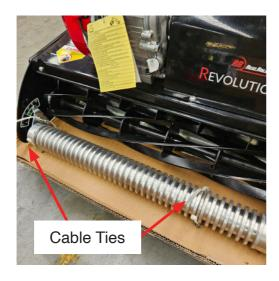
6. Loosen or cut the ties holding the front roller to the pallet. Carfully push the mower off the pallet.
