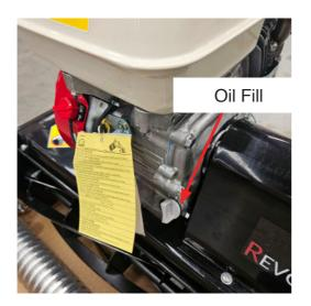
5. Fill the engine with oil as instructed in the engine manual.
